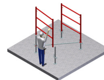
16 Remove the 2 last steel STAFLEX frames 150.
