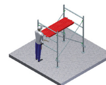
5 Position the 2 steel platform.
