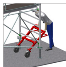
By leverage, the tower is LIFTED.
