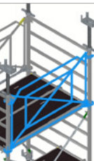
Multidynamic frame guardrail 92.5 / 150 (mixed steel/alu)
