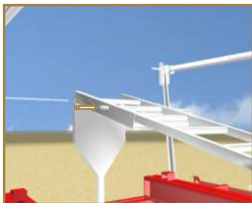
15 - Take out the ladder axis. - Assemble the step and the ladder inserting the axis into the two elements and lock with the pin \phi .
