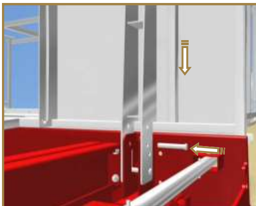
9 - Put the gangway in abutment. - Insert the pin to block the gangway. - Extend the sliding guardrails and screw the wing screws
