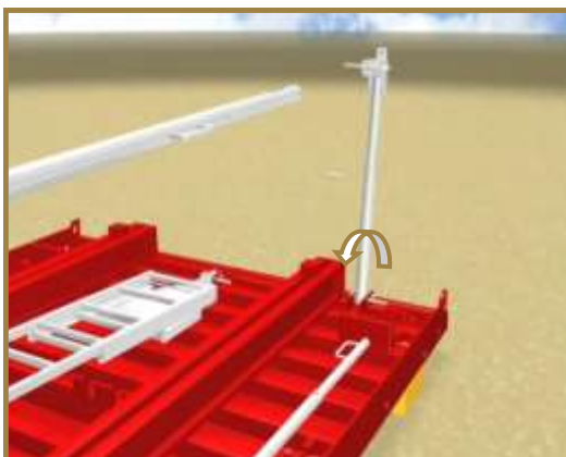
12 - Extend the struts from their packing location. - Adjust the slide length of the struts and lock them with their axes.
