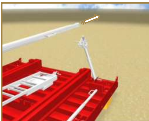
11 - Unlock the props by removing the axes. - Take out the slides from the props. - Adjust the slides according to wall formwork height and lock the props with their axes
